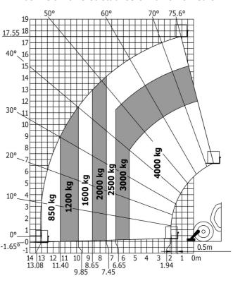
Machine on stabilisers with Man basket Metric
