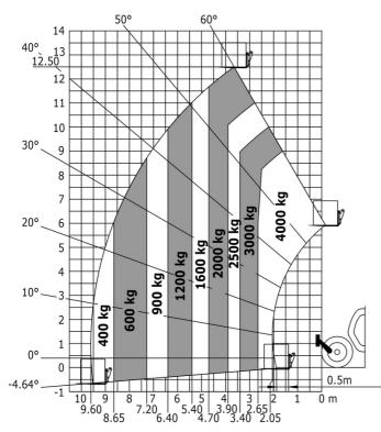
Machine on lowered stabilisers with forks Metric
